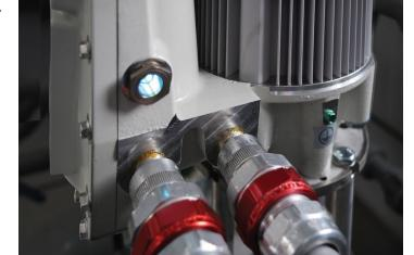
KVA38 highlighting the indicator light, conduit entry ports, and external grounding screw for easy monitoring and safety.
